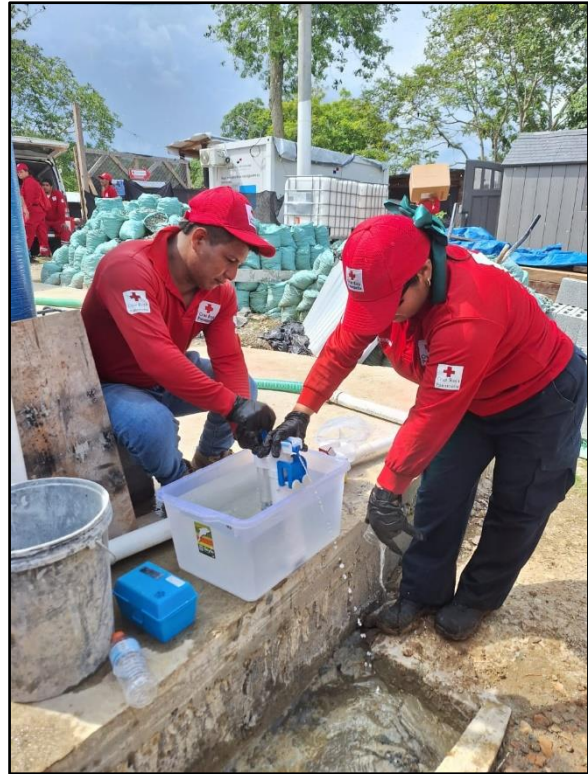
Sampling of pre-treated water with aluminium sulphate for GRIFAID filter tests (left) and subsequent practical test (right).
