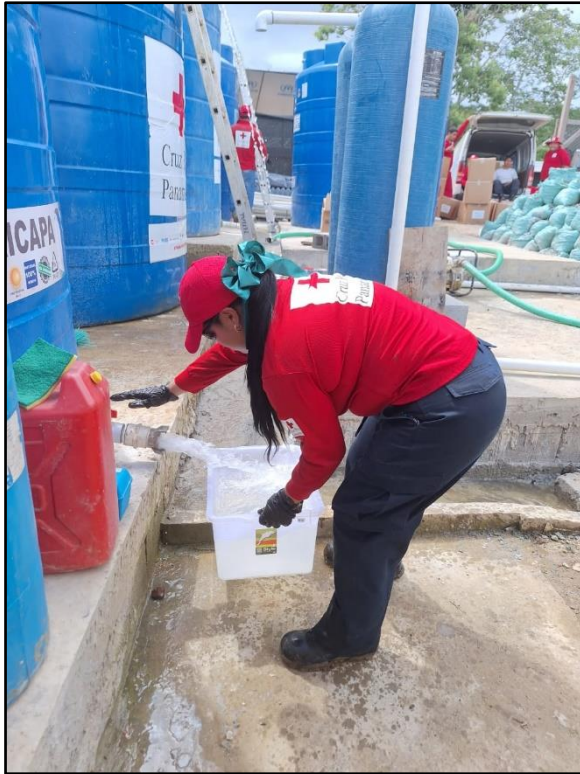
Sampling of pre-treated water with aluminium sulphate for GRIFAID filter tests (left) and subsequent practical test (right).
