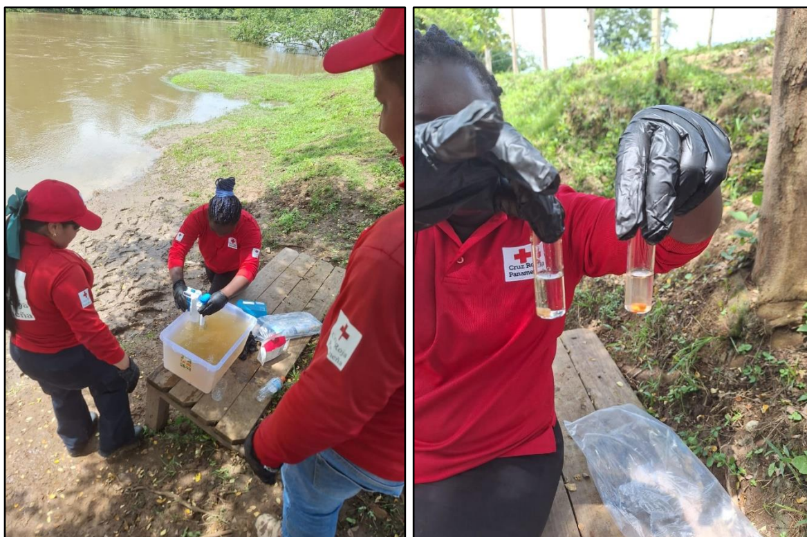
Use of GRIFAID family filter with raw water from the Chucunaque River (left) and rapid coliform tests performed on the filtered water (right).
